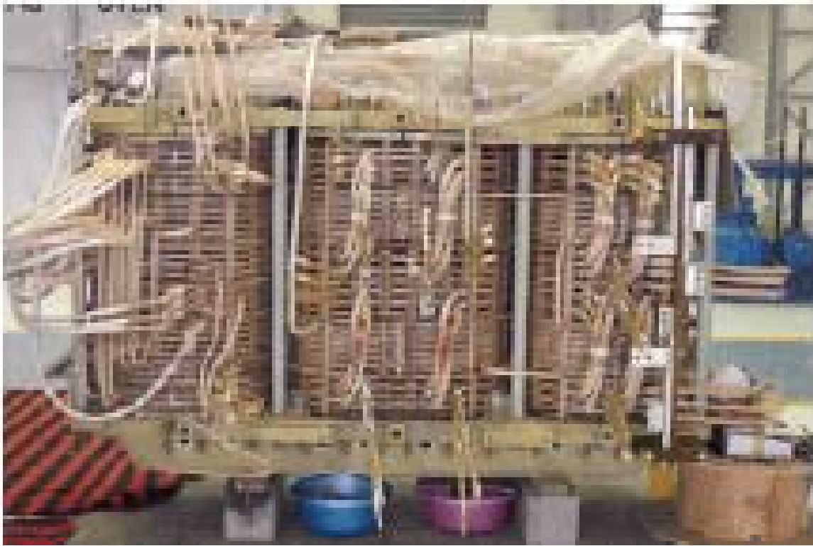
5400 KVA Loco Transformer Winding Assembly
