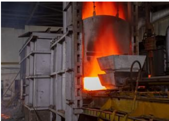
(iii) Aluminium Furnace
