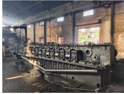
Rolling Mill with 15 Stand
