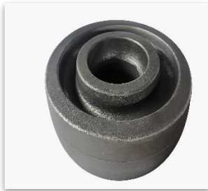
Gear component after forging stage.
