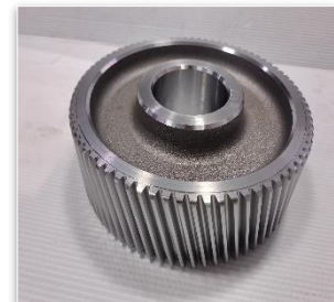
Gear component after teeth cutting process.
