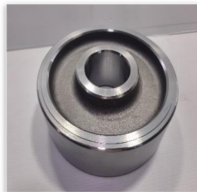
Gear component after machining stage.
