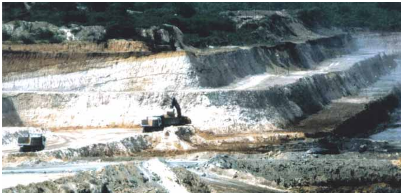
Over burden removal process in progress on bench of an Open-cast coal mine
