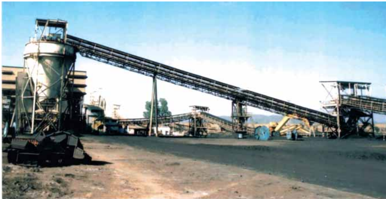
Sized Coal being transported through Conveyer Belt and stored in Coal Stacker to be washed in a Coal Washery
