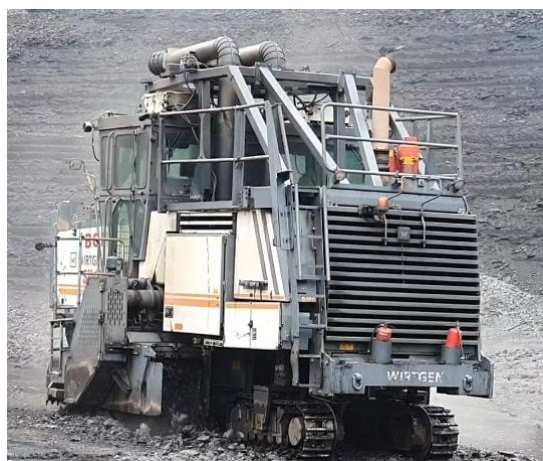
Fig. 28 - Surface miner in operation at SOCP, MCL
