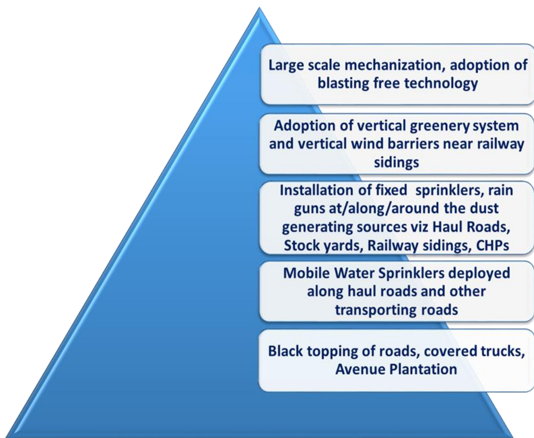
Fig. 47 - Air Pollution Control Measures
