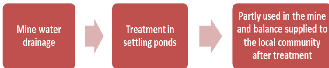
Fig. 52 - Mine water drainage system at CIL
