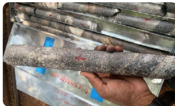
● Drill core indicating Graphite Gneiss in Arasanuru Graphite Block
