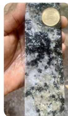
● Drill core indicated TREE value >3,000 PPM
