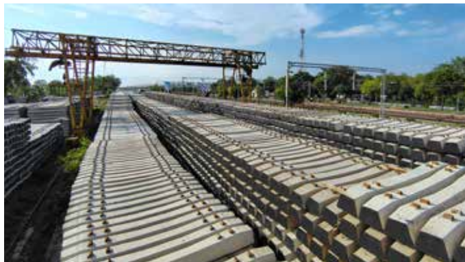
Wider Base Sleepers Confirming to RDSO Drawing No. RT-8746 Stacked on Siding Yard for Loading into Wagons/Trucks at Karari-II, in Uttar Pradesh
