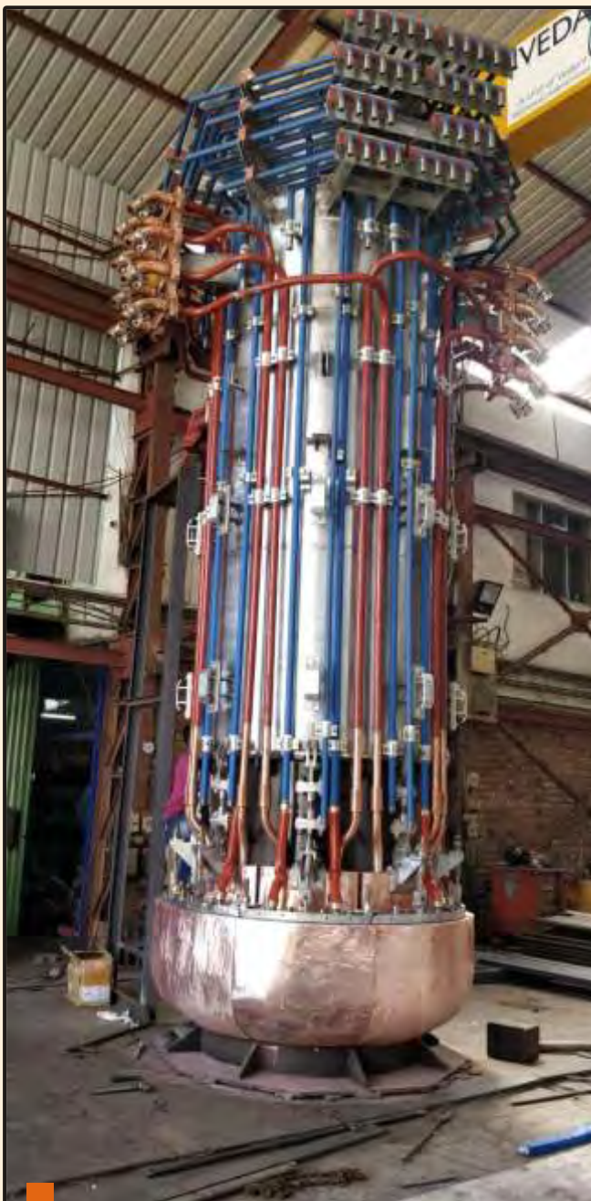
24 MVA Furnace Electrode Assembly
