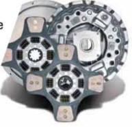
15"/380mm Single & Twin Direct Pressure Coil Spring
