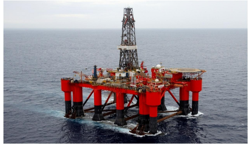
3 rd Generation Semi-submersible Rig "Essar Wildcat"
