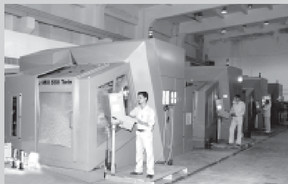
CNC 5 Axis 2 Spindle Machines installed at New Turbine Blade shop, Haridwar
