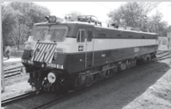
Electric Locomotive (25 kV AC, Type WAG 7)
