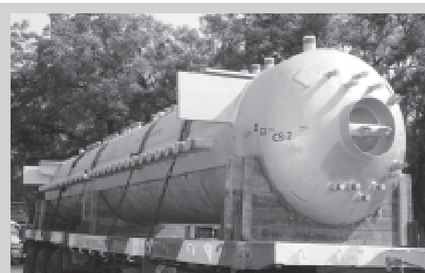
Boiler Drum (Unit-III) under dispatch for HMEI Guru Gobind Singh Refinery at Bhatinda, Punjab
