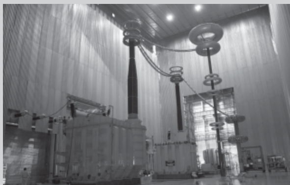
180 MVA, 1200 kV Testing Transformer & 80 MVAR, 765 kV Single Phase Shunt Reactor at UHV Lab, Bhopal
