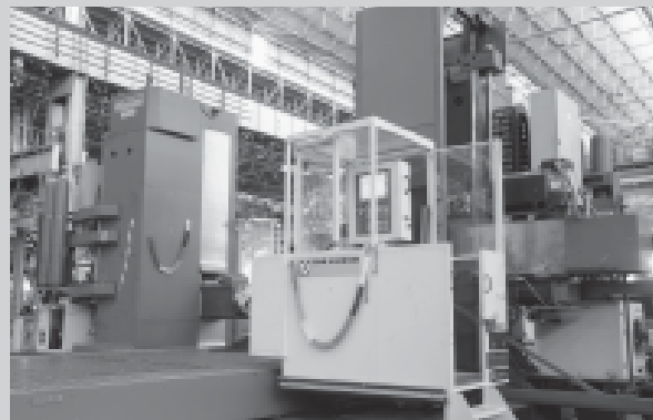
Drum U-shell edge preparation machine installed at BHEL, Tiruchirappalli
