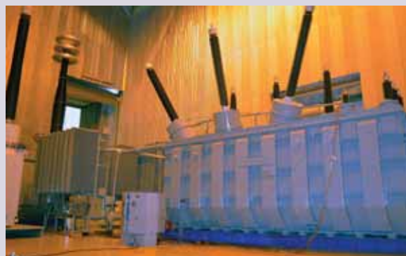
Commercialization of indigenously developed 400 kV, 315 MVA (3 Phase), Phase Shifting Transformer
