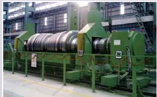
Special Purpose Fir Tree Groove Milling Machine at HEEP, Haridwar
