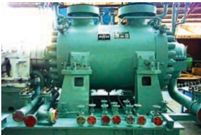
Multi-stage centrifugal compressor manufactured & supplied by BHEL
