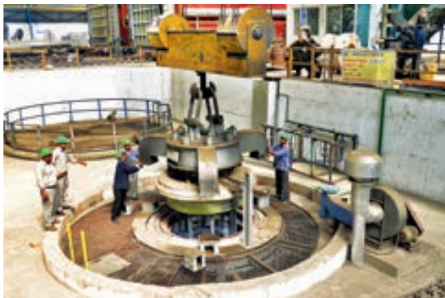
Vertical Shaft Furnace for heat treatment of more than 10M long forgings established at CFFP, Haridwar
