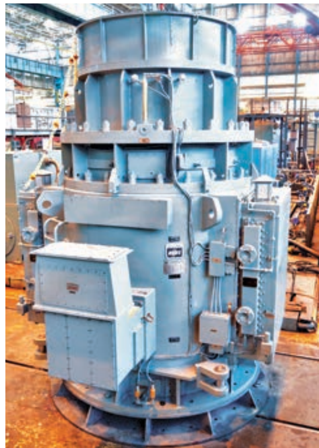
6 MW, 6.6 kV Primary Coolant Pump Motor
