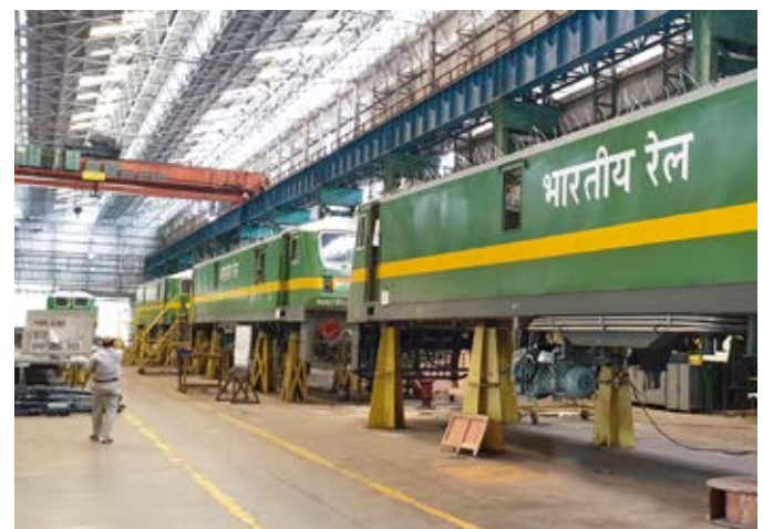
WAG9 locomotives under manufacture for Indian Railways at TP Jhansi
