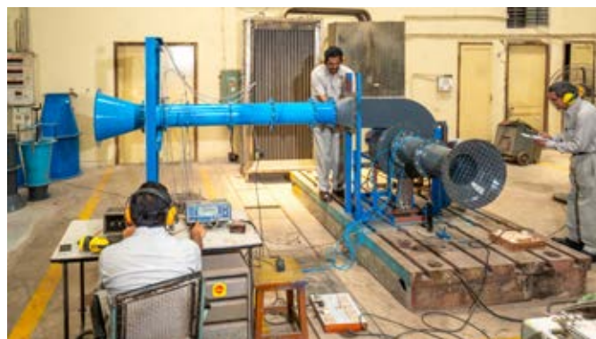
Axial fan speed and flow test facility at Corporate R&D, Hyderabad
