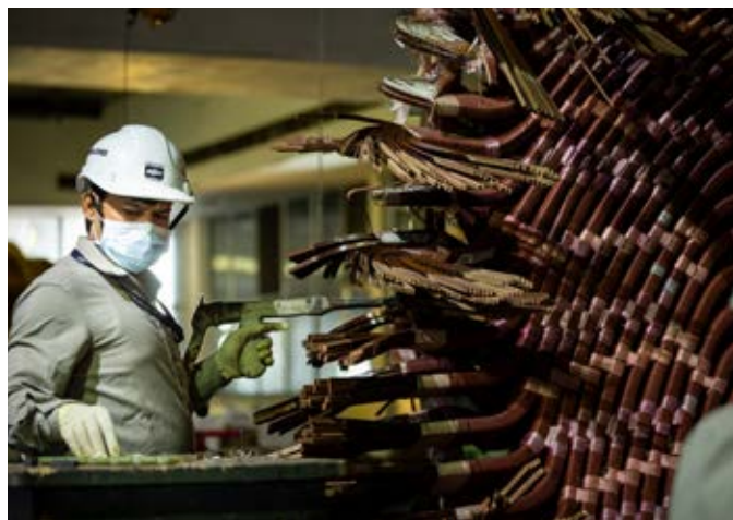
Captive plant generator winding insertion in progress at HPEP Hyderabad
