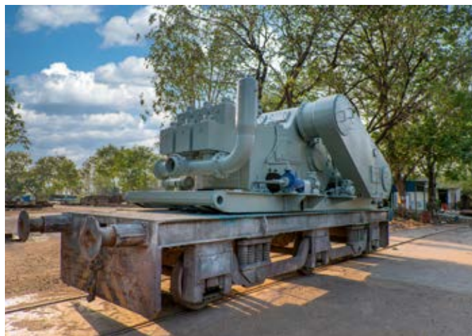
Mud pump used in oil rig system ready for dispatch at HPEP Hyderabad
