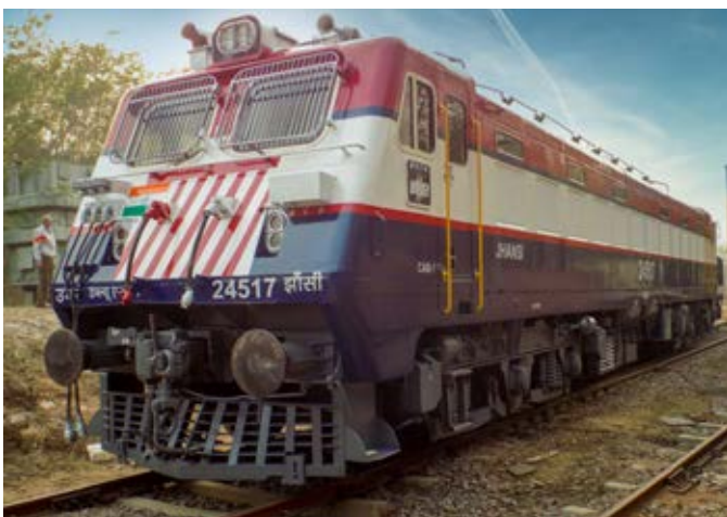
BHEL make 5000 HP WAG 7 electric locomotive with retrofitted regenerative system supplied to Indian Railways
