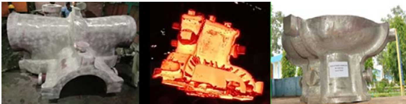
World's heaviest and largest casting in Alloy 625 grade (IP Inner Casing LH – 21 MT & UH – 9MT) for AUSC mission project manufactured at CFFP Haridwar
