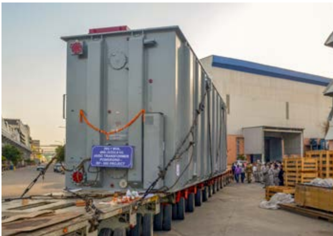
295.1 MVA, 800 kV, HVDC CONVERTER TRFR for 800 kV Class Single phase HVDC Converter Transformer being despatched from HEP Bhopal
