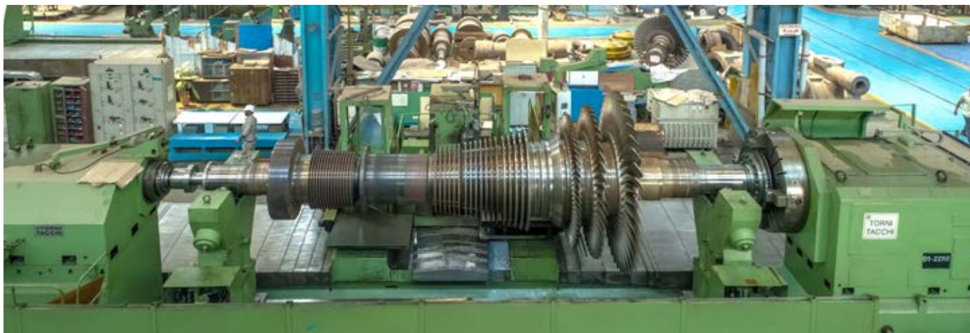
Highest rating 150 MW IP turbine for captive plant applications at under testing at HPEP Hyderabad
