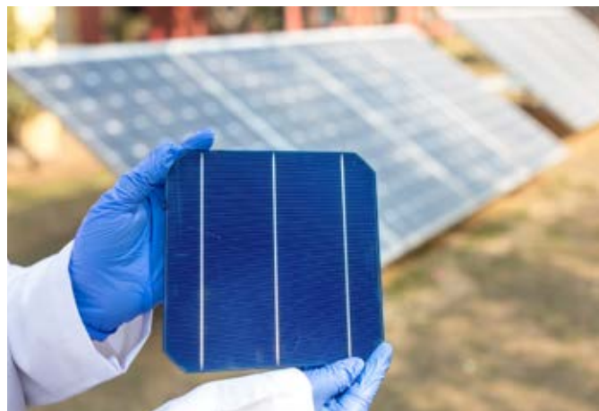
Prototype high efficiency solar cell using PERC technology under development at BHEL ASSCP, Gurugram
