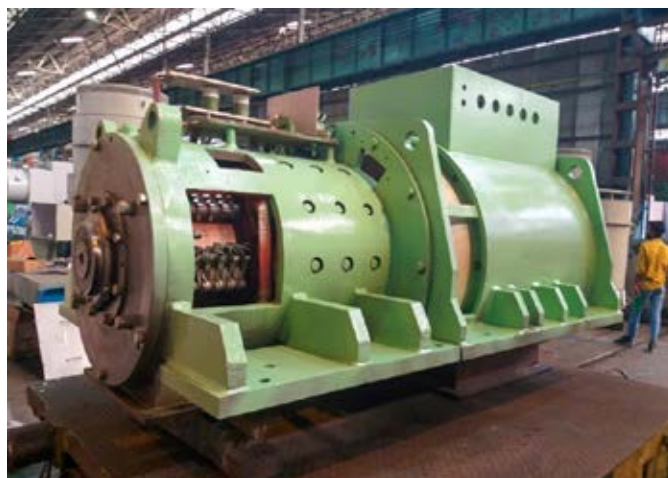
500 kW Main Motor Generator (MMG) (assembly of AC & DC machine) set for defence application designed & manufactured by BHEL
