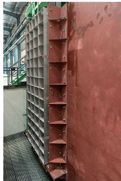
Open Channel Gate for Dalmarnock WWTW Scottish Water, UK
