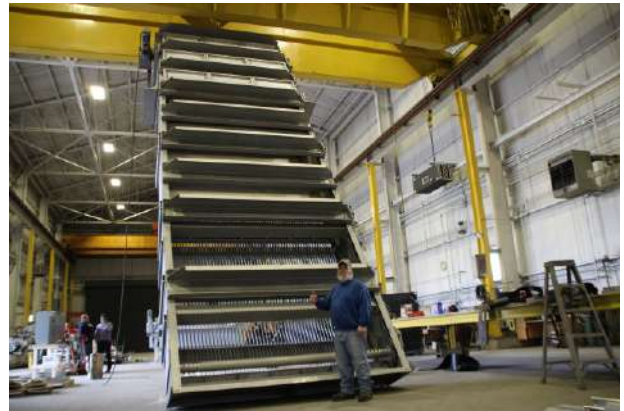
Multirake Bar Screen for Port Monmouth, Orange, USA
