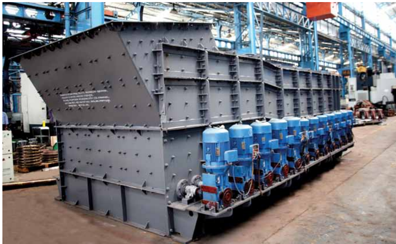
Individual Drive Roller Screen Supplied To Flsmith Minerals Ltd. For Utkal Almina Project.
