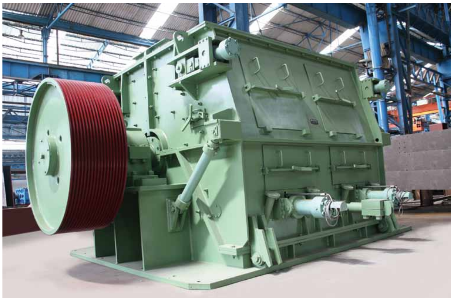
Fully Automatic Reversible Hammer Crushers, (Rate 500 T Per Hour), Supplied To Posco E &C, South Korea For (-)3 mm Product
