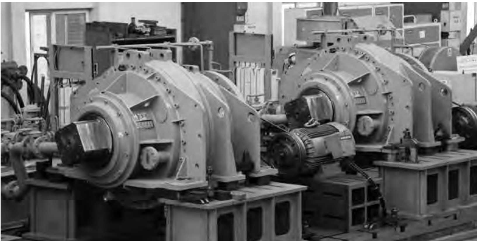
▲ Factory testing of Sugar Mill Drive Planetary Gear boxes
