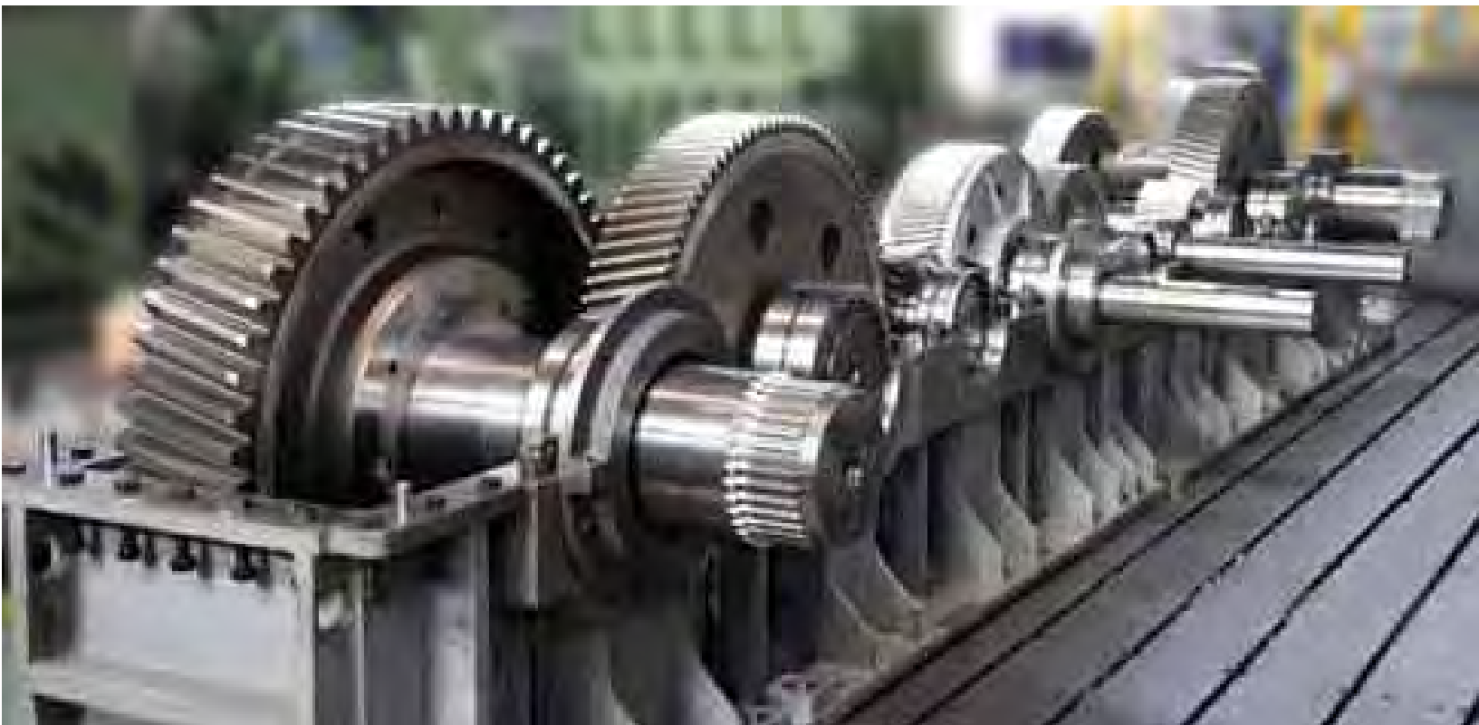
▲ Main Hoist Drive Gearbox for Hot Metal Ladle Crane
