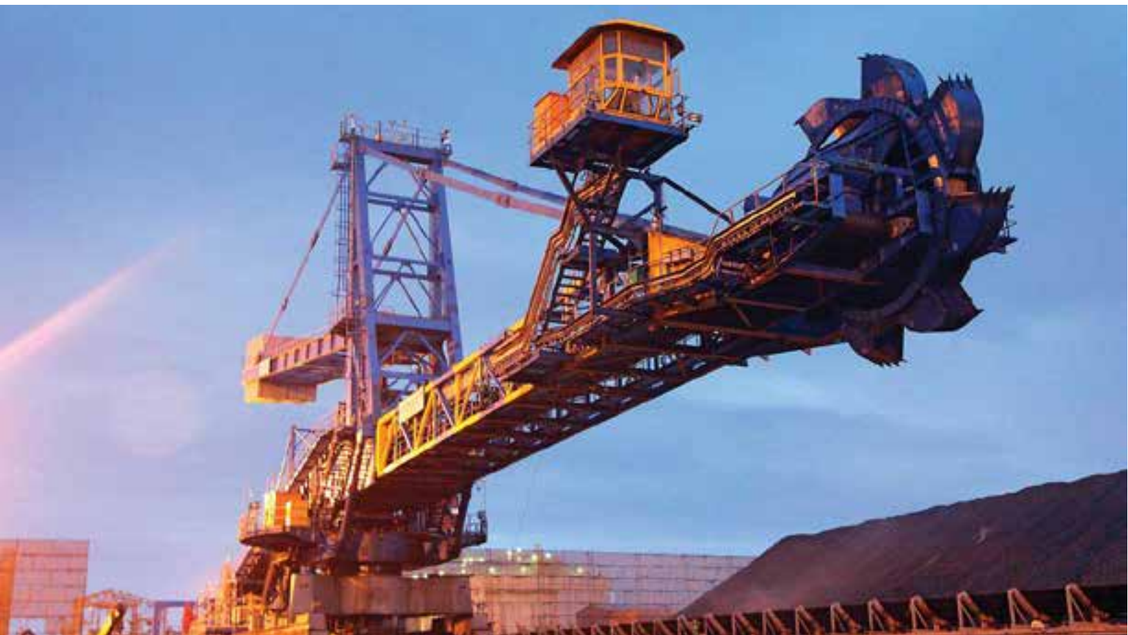
▲ Combined Stacker cum reclaimer at Adani, Dahej Port (4200 TPH Stacking/2500 TPH reclaiming, 41 M boom)
